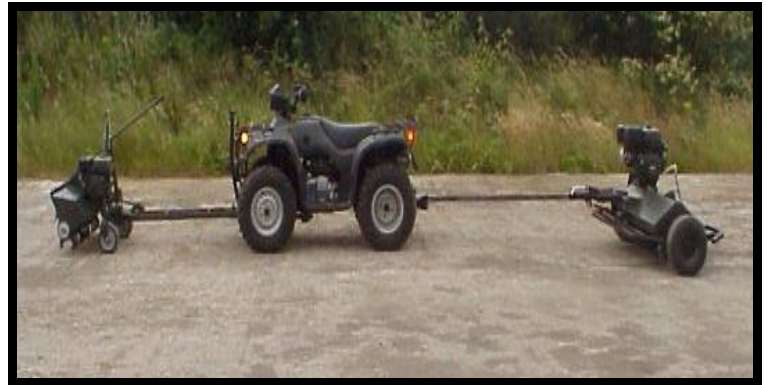
Fig 5. THRASHER, wheeled mine-clearer (KentreeLtd, IR)
