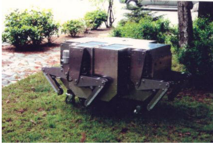
Fig 1. The AMRU-3 electro-hydraulic driven six-legged robot
