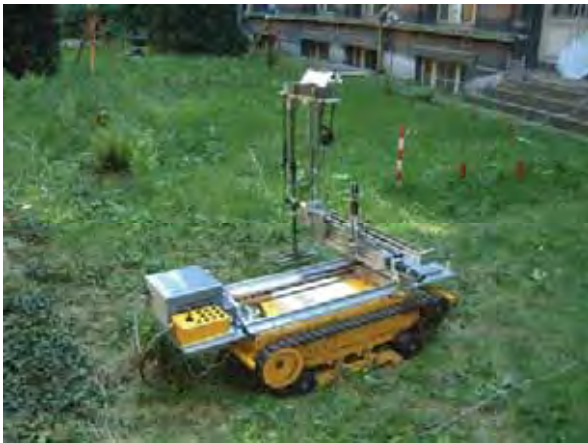
Fig. 11. The Hunter platform with the Cartesian scanner
