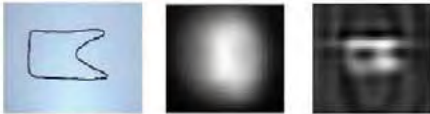
Fig. 22. Close-loop wire (left), the raw metal detector image (centre) and the image after image processing (right).
