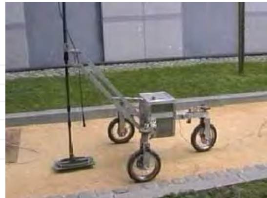
Fig. 1. The Tridem equipped with a metal detector mounted on a passive boom.
