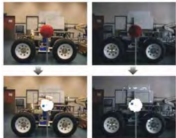
Fig. 15. Illustration of the colour constancy in different illumination conditions.
