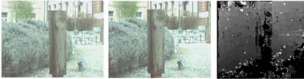
Figure 2: Image motion field of right camera: a) Image at t_{i-1} ; b) Image at t_i ; c) Image motion field
