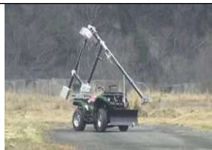
Fig 6.a. Gryphon-IV remote maneuvering experiment. The system can be remote-controlled in a range of about 150meters. Tokyo Institute of technology, JP [8]
