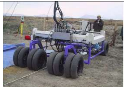
Fig.6.d. 16-wheeled (each tube tire able to support about 25 daN without explosion –most sensitive AP-mine is 0.064 bar) Sensing Vehicle, Tohoku University, JP [10]
