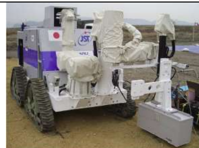
Fig.6.f. Mine Hunter Vehicle, equipped with a teleoperated hydraulic manipulator, Chiba University, JP [12]
