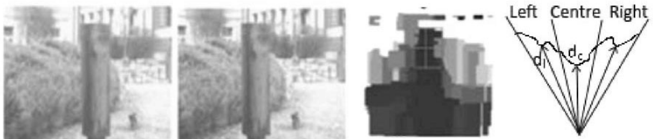
Fig. 1. Stereo Processing a) Left camera image; b) Right camera image; c) Dense depth map (white=far, dark = near); d) Depth line with nearest distances to obstacles on the left, in the middle and on the right.
