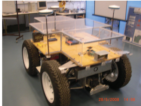
Figure 1. The RobuDem platform with GPS and stereo vision system, used for evaluating the presented algorithms.
