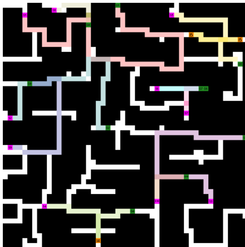
Figure 9: A map with small passages. Cooperative A* was used to generate the paths for the robots. This map has covers where robots can wait to let other robots pass to avoid collisions.
