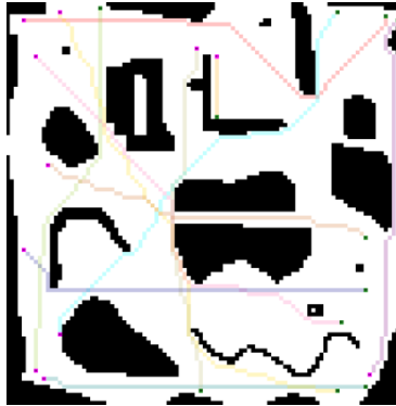
Figure 13: Binary map with equal traversability in the free space region. The paths are calculated without taking into account the distance transform information.
