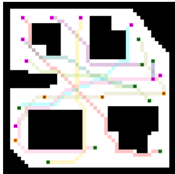
Figure 8: Typical results of path planning with the cooperative A* algorithm.
