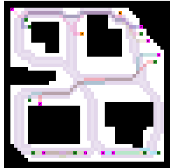
Figure 19: Multiple Voronoi lanes are used to allow robots to pass each other. In this figure 3 lanes are shown. The middle one will be preferred when planning the robots paths.
