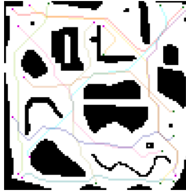
Figure 14: The paths in this map are calculated while incorporating the information available from the distance transform of the map, resulting in paths further away from the obstacles.
