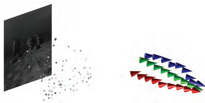
Figure 6.8: Estimated 3D sparse feature points and camera views for the synthetic sequence. (green = ground truth; red = three-view motion estimation; blue = after bundle adjustment)
