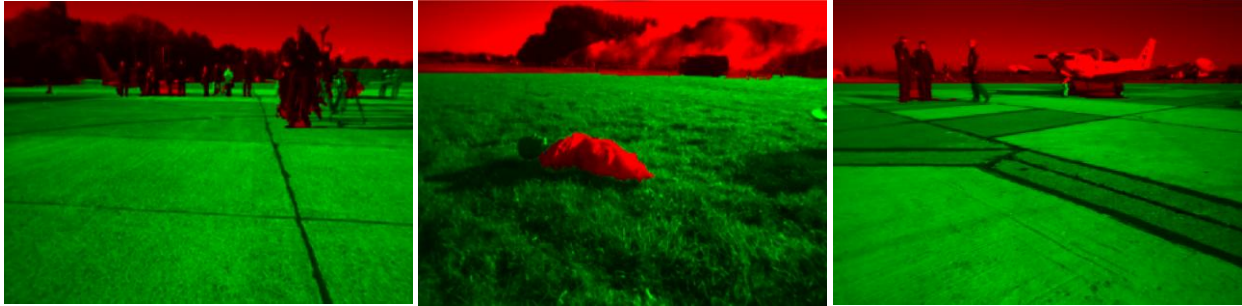
Figure 1: Terrain Traversability Estimation Results (green = traversable; red=obstacle)
