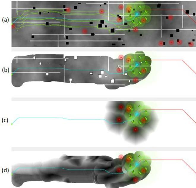
**Fig. 12:** Snapshot of the mission during execution. In blue the traversed path is shown, in red the current global planned path which changes continuously when new information comes in. (a) The map information, and intruder locations. (b) The information gained by the robot team about the environment at this stage of the mission. (c) The distance transform map of the intruders that are currently in view. (d) Distance transform map in convoy memory used to update the path.
