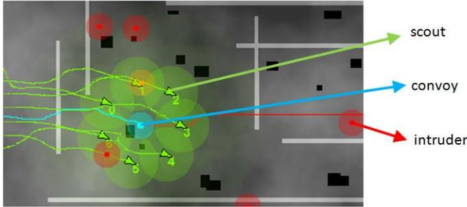
**Fig. 4:** Screenshot of the simulation: convoy, intruders and scout and their respective sensor ranges. The scout robots try to maximize their information gain by forming a circular formation around the convoy.
