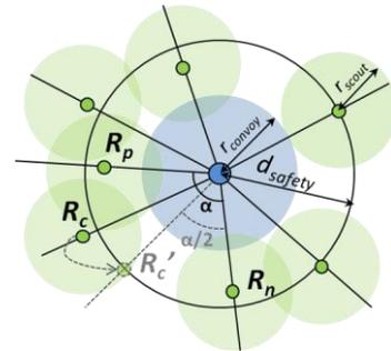
**Fig. 5:** Every scout robot will adjust its speed  $v$  and angular speed  $\omega$  to move towards its next goal position. This goal position is calculated by looking at the previous and next neighbor  $R_p$  and  $R_n$  of the current robot  $R_c$ . The new goal position  $R_c'$  is at a distance  $d_{safety}$  from the convoy and lies on the angle bisector of the angle  $\alpha$  between  $R_p$  and  $R_n$ .
