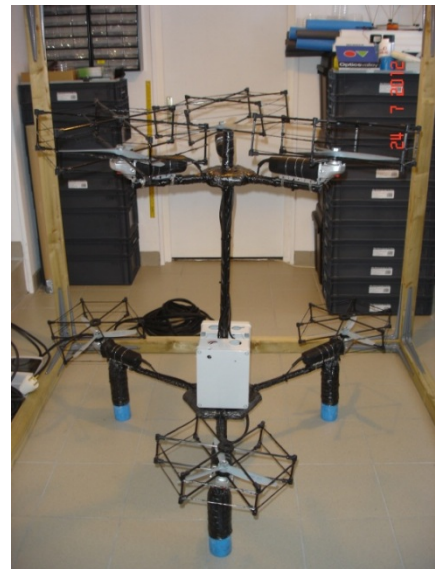
FIG. IV – Very first prototype of GyroPendulum MineMarking Platform 220v AC with Umbilical Cable
