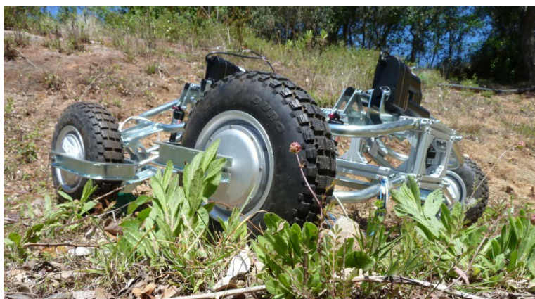
Figure.3 ISR-TT all terrain robot for stand-off and close-in detection of ED (under construction).
