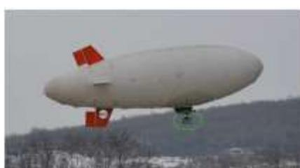
CTDT Airship for hyperspectral data acquisition in Croatia [16]
