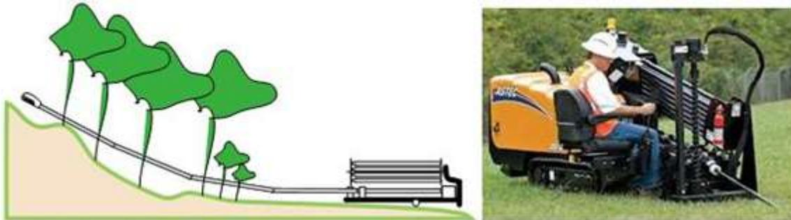
Figure 6. Schematic of the automatic REST sampling method (left), and example of drilling machine used as reference for the development of the REST system (right)
