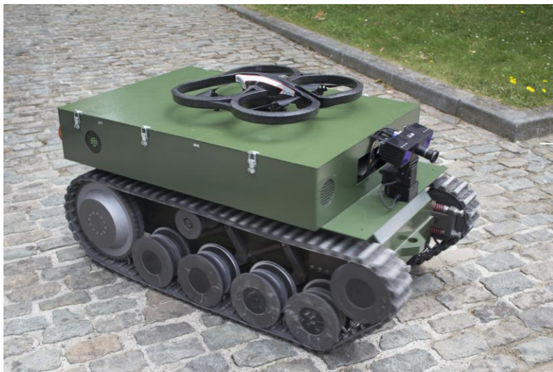
Figure 1: The system setup, consisting of the UGV tEODor base, UAV and an integrated active Time-Of-Flight Depth sensing system
