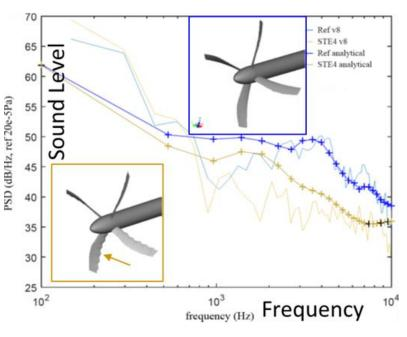
Building on previous expertise and inspiring from biology, specific shape determining parameters have been identified as yielding potential noise reduction while maintaining high efficiency and structural integrity.
