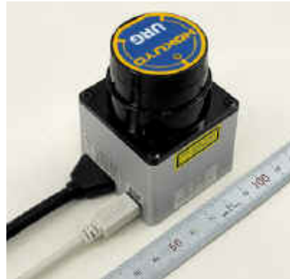
(d) Hokuyo URG Laser Rangefinder: Range 4m, Accuracy \pm 10 mm, Field of view 240 degrees, Angular resolution 0.36 degrees, Max scan rate 10 Hz, Power 2.5W, Weight 0.16 Kg
