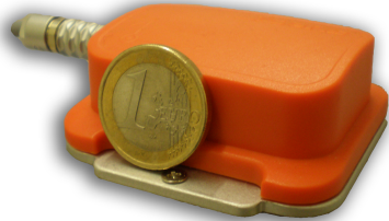
(c) XSens MTi IMU device: accurate full 360 degrees 3D orientation output (Attitude and Heading), highly dynamic response combined with long-term stability (no drift), 3D acceleration, 3D rate of turn and 3D earth-magnetic field data, high update rate, temperature, 3D misalignment and sensor cross-sensitivity compensated
