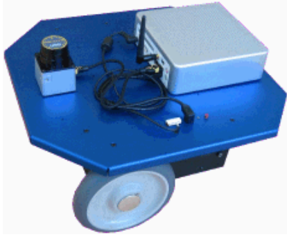
(a) Mobile platform Erratic: H8S controller, Servo and analog/digital I/O, 2x 75W motors, 500 CPR encoders, IR floor sensors, 3x 7A 12V batteries. Onboard PC: 1.4 GHz Celeron, 802.11b/g, USB 2.0, IEEE 1394b, 40 GB, 512 MB
