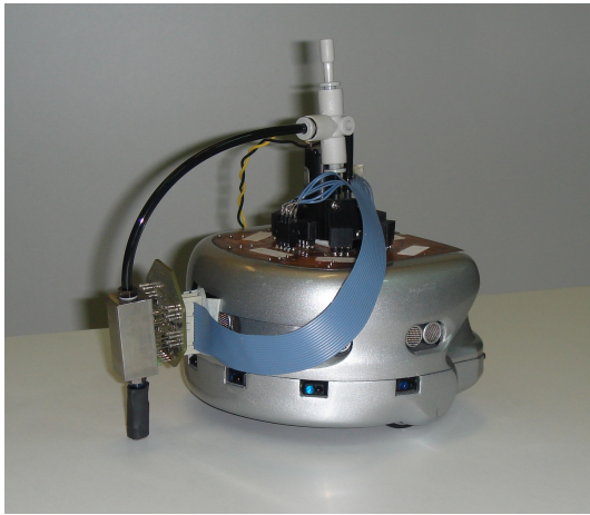
Fig. 1. Picture showing a Khepera III robot with a chemical trail detection olfactory system.
