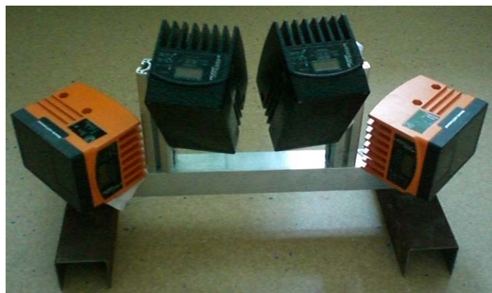
Figure 2: 3D local navigation sensor system based on 4 3D PMD sensors.
