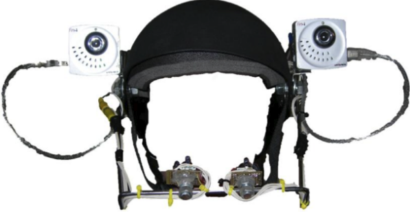
Figure 5. The gaze-machine used to acquire the scanpath.
