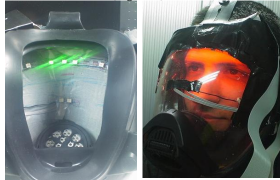
Figure 4 Light Array Visor [LAV2] using real fire fighting helmet.
