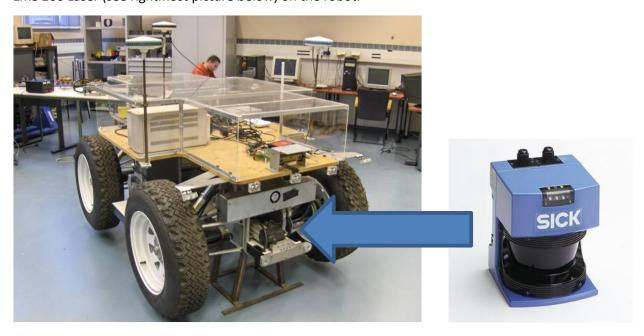
The Laser system will of course also need to be controlled, such that data can be retrieved from the Laser system, such that it can be analyzed. As a first application with this Laser, we want to detect whether the terrain in front of the robot is traversable or not, based on the Laser Data.
