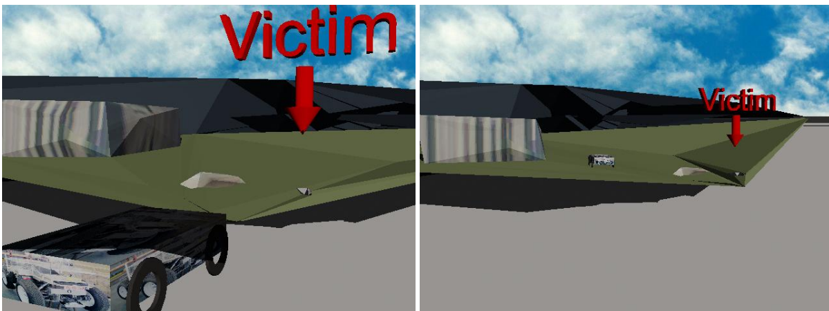
Figure 6: Reconstructed 3D model of the environment, showing the camera/robot position and an indication of the presence of human survivors
