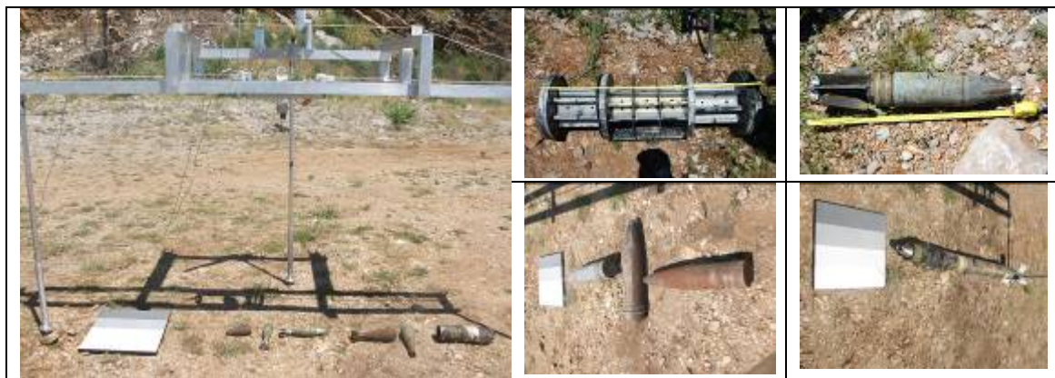
Figure 13. Measurement of the coefficient of reflection by line scanner. Different types of UXO have been measured.
