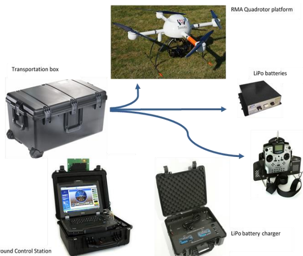
Figure 2 Microdrones MD4-1000 quadrotor with field control base station
