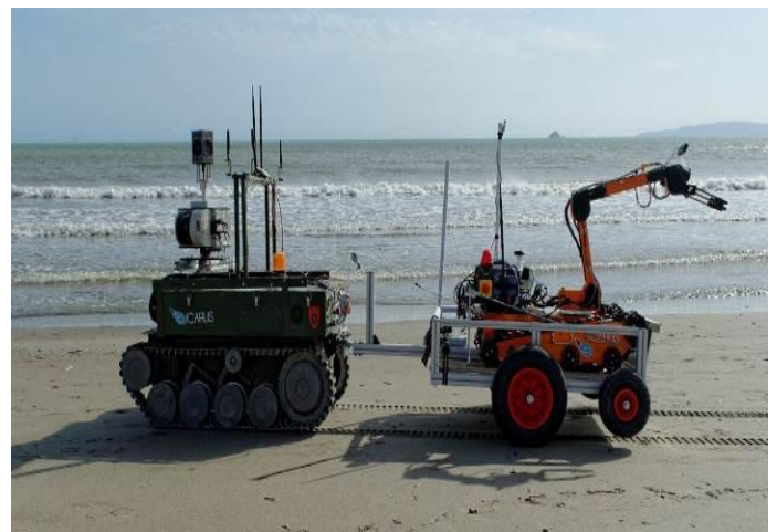
Figure 9 - ICARUS team land components: TEODOR (the green tracked vehicle), and SUGV (the orange vehicle in the trailer).
