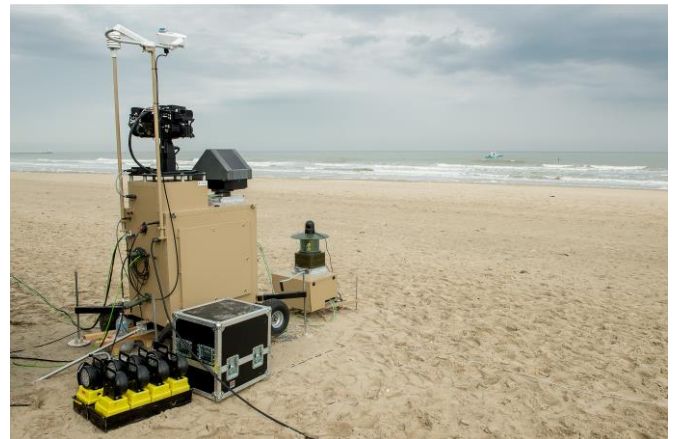
Figure 2: SafeShore drone detection system installed on the beach in Belgium during the SafeShore North Sea trial Picture by Daniel Orban
