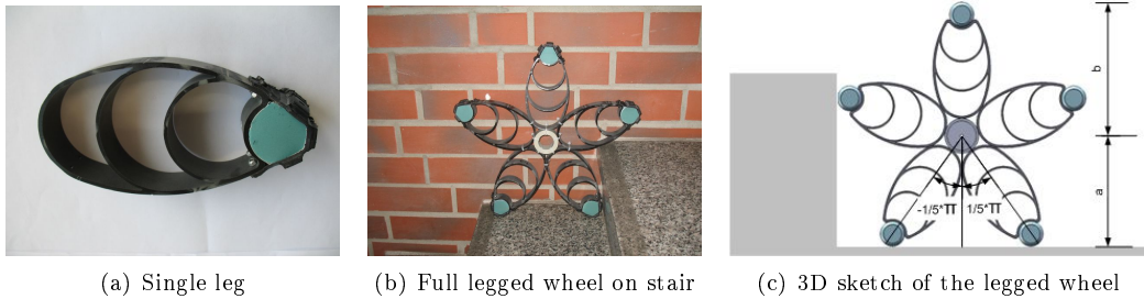
Figure 3: Design of the legged wheel
