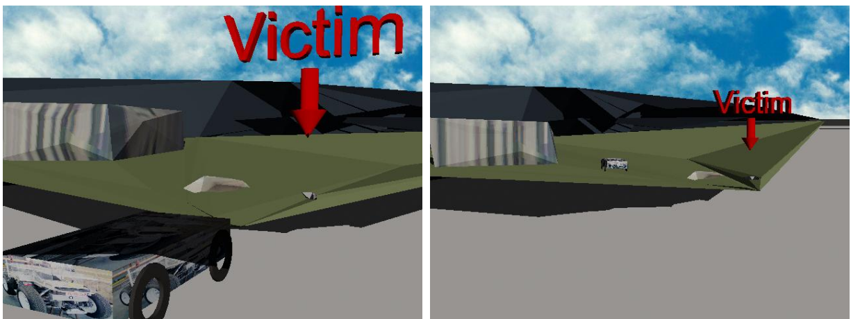
Figure 3: Reconstructed 3D model of the environment, showing the camera/robot position and an indication of the presence of human survivors, by fusing the 3D information with the output of a human victim detector algorithm [1].
